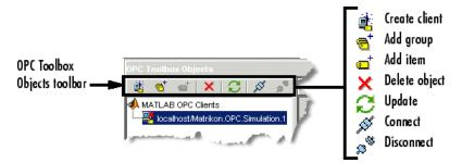
Click **Connect** in the **OPC Toolbox Objects** toolbar. If the client is able to connect to the server, the icon for that client in the **OPC Toolbox Objects** tree will change to show that the client is connected. If the client could not connect to the server, an error dialog will show any error message returned. See "Troubleshooting" on page 1-22 for information on why a client may not be able to connect to a server.
